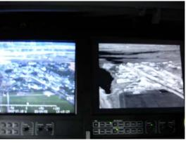
the crew all have their hands full doing the rescue). The appearance of the aircraft has changed slightly with the new equipment: the turret dangles from the bottom of the port fuselage, just inboard of the undercarriage, and the radar cabin has been refitted with the single original radar display giving way to two new screens, each of which can display either the radar picture, the IR
